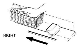
At the end of the cut, position your hand on TOP NEAR THE END of the work piece and continue feeding the work piece until the cutter guard has returned to its closed position.
